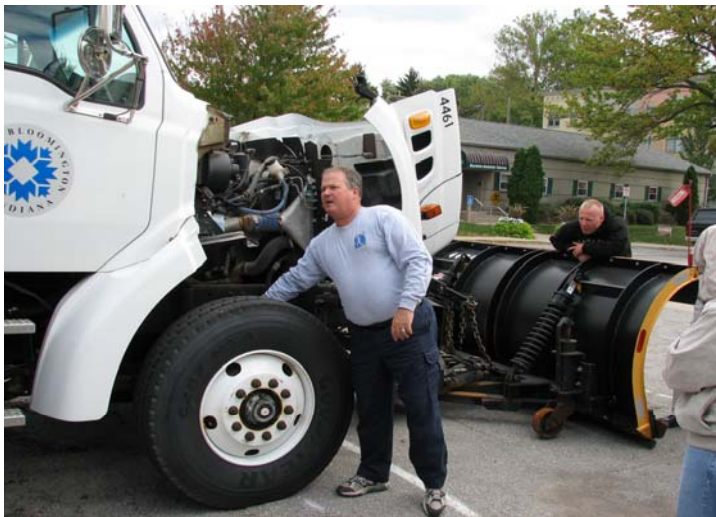
Instructor James Jackson shows students the brake chamber on a Bloomington City Street Department truck during the afternoon CMV inspection demonstration. Ironically, the truck was found to have an air leak which required repair before it could be legally moved.
