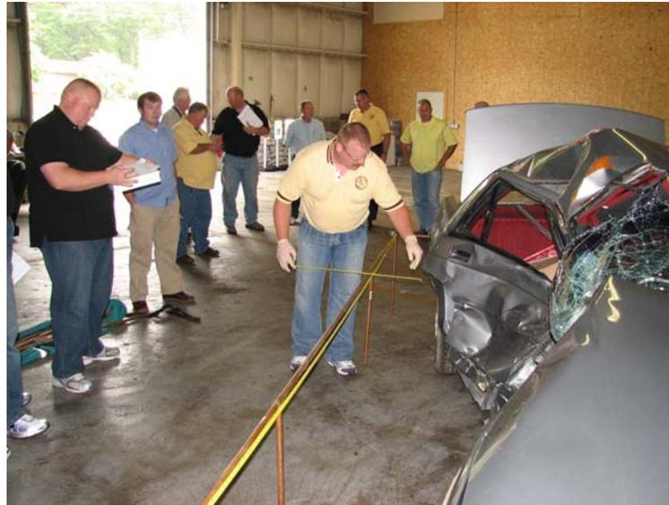
IACAI North Director Phil Nott demonstrates a method of obtaining crush measurements on one of two vehicles provided for the Vehicle Damage Analysis seminar held at the Warsaw Police Dept., on June 17th.
