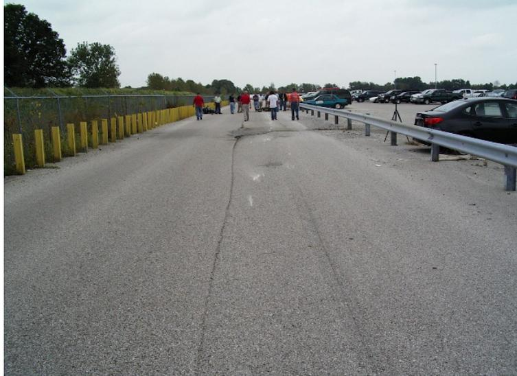
A long combination of scratches and gouges points the way to the final rest of one of three motorcycles tested during the Motorcycle Crash Investigation seminar recently held in Plainfield.
